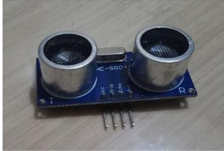
**Gambar 3.9** Sensor Ultrasonik
