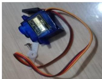
**Gambar 3.11** Motor Servo DC
