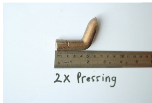
Gambar C.2 Aluminium Zircon 2 Kali Pass Penekanan ECAP-PC
