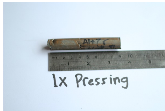
Gambar C.1 Aluminium Zircon 1 Kali Pass Penekanan ECAP-PC
