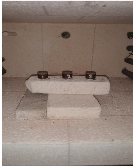
Gambar 3.5 Sampel Diproses Age Hardening
