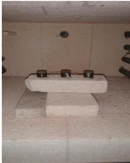
Gambar 3.5 Sampel Diproses Age Hardening
