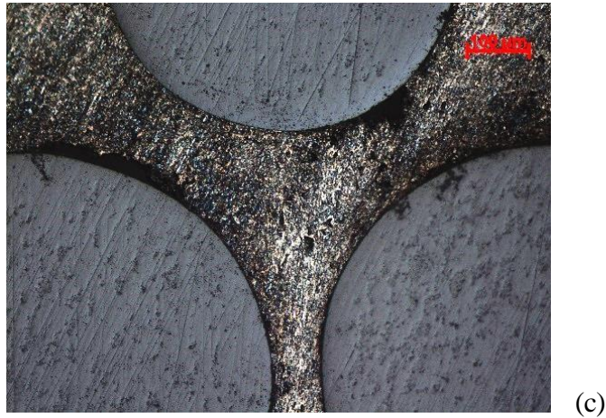
Gambar 4.9 Struktur Mikro Perbesaran 100x (a) Sampel Non Heat Treatment 1 Siklus (b) Sampel Non Heat Treatment 2 Siklus (c) Sampel Non Heat Treatment 3 Siklus
