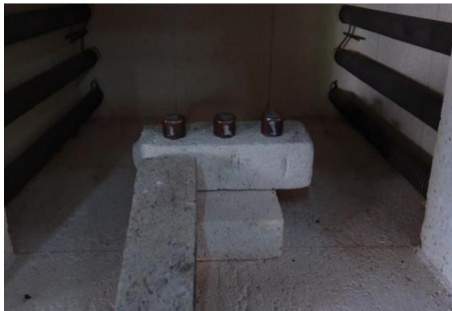
Gambar 3.4 Sampel Diproses Annealing
