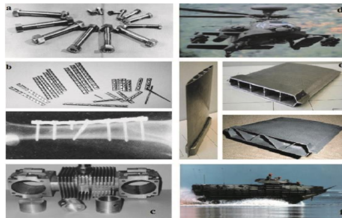
Figure 5. Application areas of ECAP and ARB: (a) high-strength thread developed in Russia (b) plate implant made of SPD nanostructure developed in Europe (c) engine block machine made of AA1420 nanostructure developed in Russia (d) military helicopter body of high-strength material developed in collaboration by Russia Europe and the UK (e) UFG Ti-6Al-4V superplastic sheet material for Hollow blade model developed by Japan and several European countries (f) military device - amphibious assault vehicle, belonging to BAE Systems developed by a joint project between Russia, USA, Japan and England.
