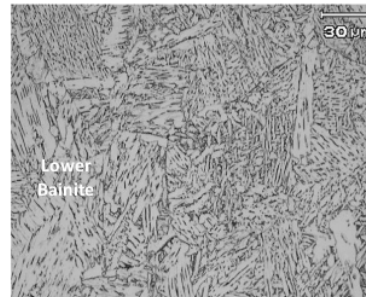
Fig. 5a. Microstructure of Weldment at 0.75 kJ/mm of Heat Input.
