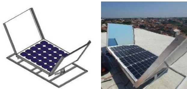
Figure 2. Solar Panel Framework and Reflectors
