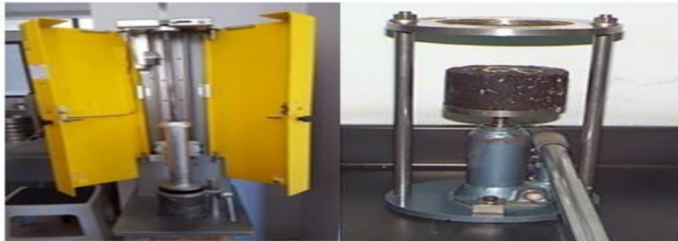
Figure 7. Marshall Testing Device with modified asphalt sample.
