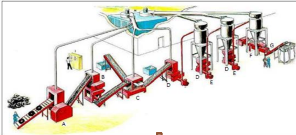
Figure 1. Recycling Technology of the waste tire. A) preliminary shredder, B) granulator, C) steel separation and textile fibres remover, D) complete cleavage, E) pneumatic transportation, F) wind-sifter, G) secondary magnetic separation and H) fibres and dust removal [5]
