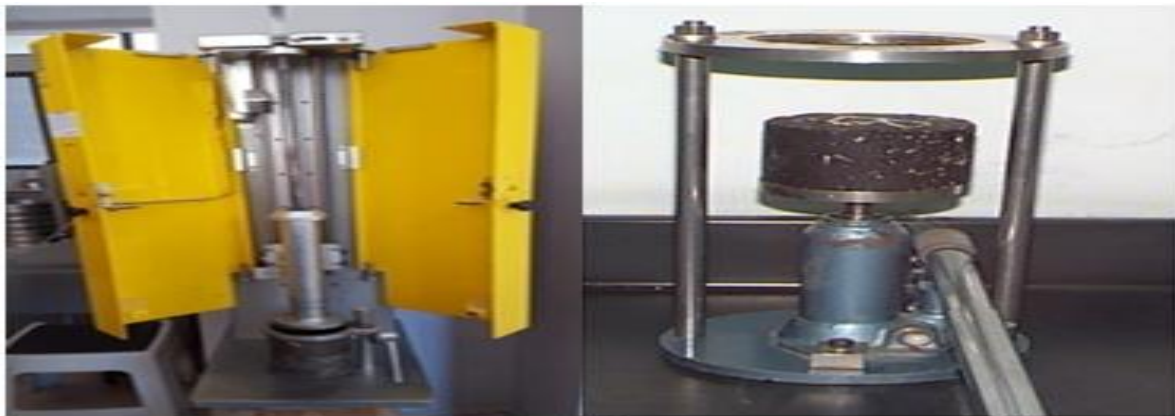
Figure 7. Marshall Testing Device with modified asphalt sample.
