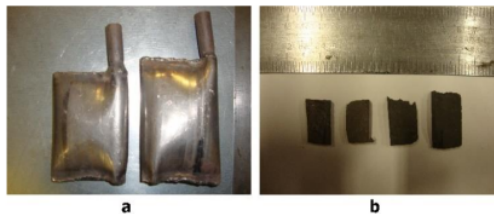
Figure 1. a). Dies of powder compaction; b). SHS solid powder
