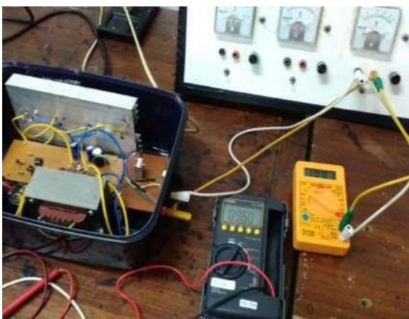
Fig. 3: The Tests DC-DC Converter Using Power Supply
