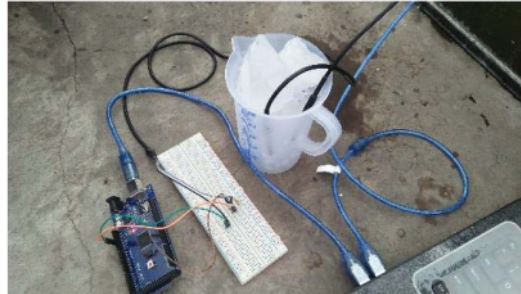
FIGURE 5. Testing of DS18B20 Sensor with Comparative Sensor at Green House
