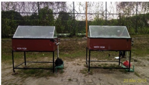
Fig. 2. Solar distillation system without PCM and with PCM
