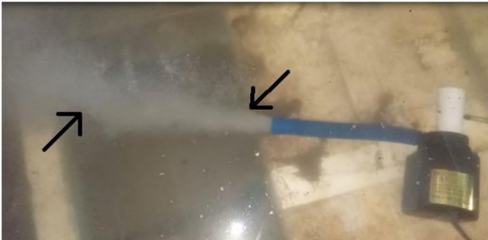
Figure 2. Air bubbles were generated from the venturi and water pump with a modified needle wheel shape (arrow) (Photograph by Herjayanto).
